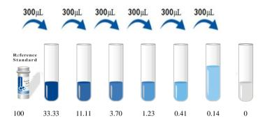
4. **HRP Conjugate working solution:** HRP Conjugate is HRP conjugated avidin.Calculate the required amount before the experiment (100  $\mu$ L/well). In preparation, slightly more than calculated should be prepared. Centrifuge the Concentrated HRP Conjugate at 800×g for 1 min, then dilute the 100×Concentrated HRP Conjugate to 1×working solution with HRP Conjugate Diluent.
