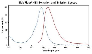
Ex:495 nm; Em:520 nm; Laser:488 nm; Filter:530/30
